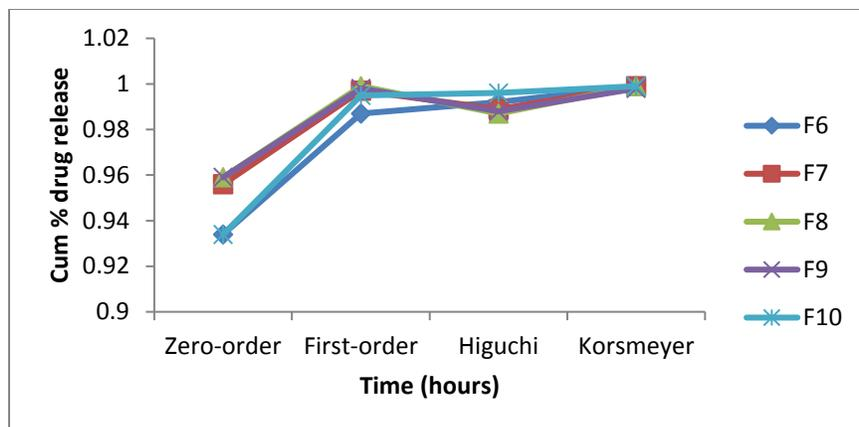
**Fig. 9: Mathematical modelling and drug release kinetics of HPMCK100M and Ethyl cellulose matrix tablets**
