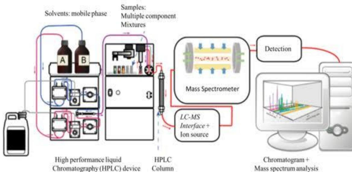
**Fig 1: Direct electron ionisation Liquid Chromatography-Mass Spectroscopy**
