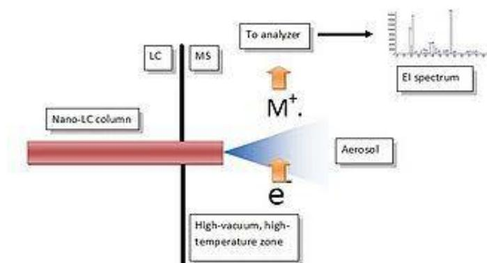
**Fig 2: Mechanism (LC-MS)**
