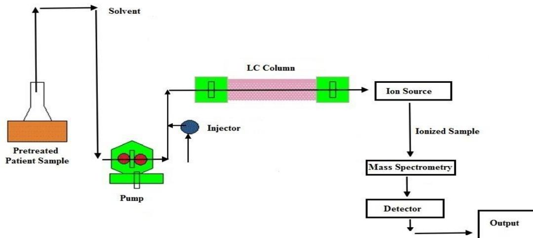
**Fig 3: Principle-Liquid Chromatography-Mass Spectroscopy (LC-MS)**
