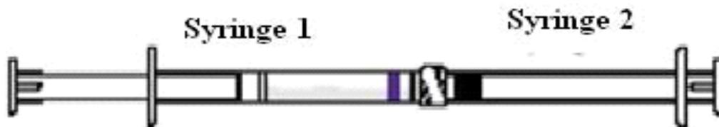
**Figure 2.(b) Couple Syringe 1 (liquid delivery system) and Syringe 2 (drug powder).**
